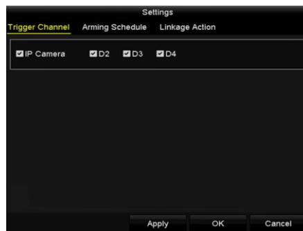
Figure 4-17 Set Trigger Camera of VCA Alarm
